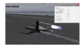
The flight model was flown in a real time simulation software with X-plane and it is shared with the STK (System Tool Kit) through a C# interface specially designed using the UDP protocol
